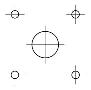
Use a 4mm or #22 drill bit for the four small holes, and a 14mm or 9/16" drill bit for the large center hole.
